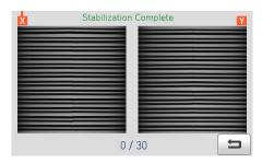
vi. After completing the Electrode Stabilize, ARC Calibration should be performed separately.
